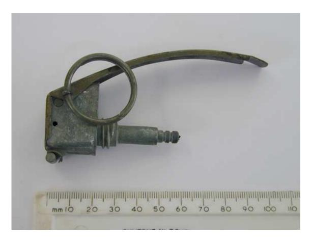
Figure 18: The lower photograph depicts a close view of grenade fragment. The top photograph depicts the grenade igniter set referenced in section 5.6 of this report.
