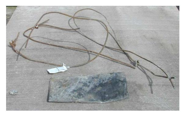
Figure 19: This photograph depicts the reinforcement bars, which were tested for the presence of explosive residues.
